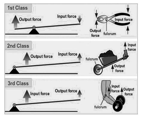
These classes are described by the mnemonic "fre 123" where the fulcrum is in the middle for the 1<sup>st</sup> class lever, the resistance is in the middle for the 2<sup>nd</sup> class lever, and the effort is in the middle for the 3<sup>rd</sup>.
