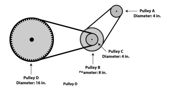
A belt and pulley system is characterized by two or more pulleys in common to a belt. This allows for mechanical power, torque, and speed to be transmitted across axles. If the pulleys are of differing diameters, a mechanical advantage is realized.
